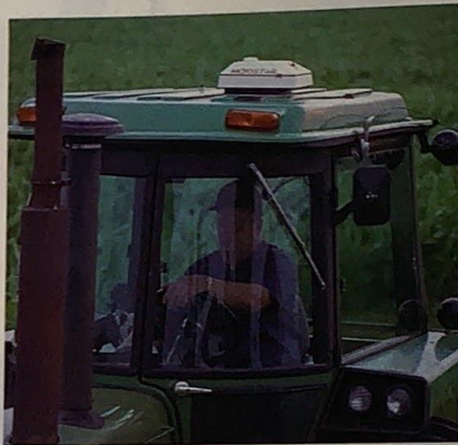
▲ TRACTOR TECH: The roof-mounted global positioning system allows fine-tuned farming.
